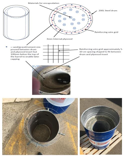
Figure 73: Diagrams and photos showing inner liner with reinforcing metal and final concrete finish in the drum
