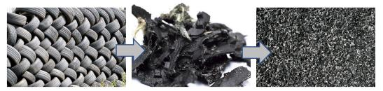
Figure 52: Waste tyres shredded and processed to granules
