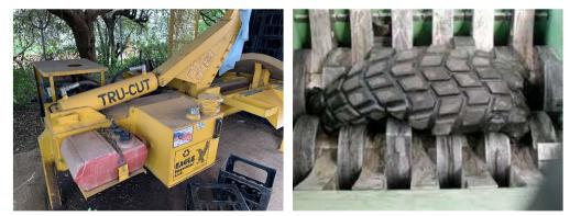
Figure 51: Tyre cutter and shredding tyres
