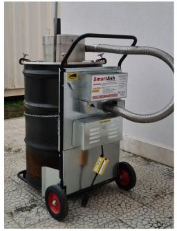
Figure 6: Solid waste, biomedical and barrel incinerator with air induction
