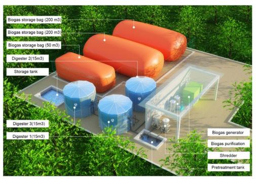
Figure 18: Examples of small to large scale biogas recovery systems
