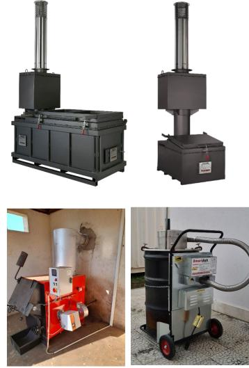
Figure 76: Solid and biomedical waste and barrel incinerators
