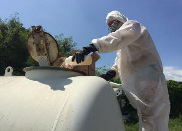
Figure 72: Alkaline hydrolysis treatment for waste pesticides
