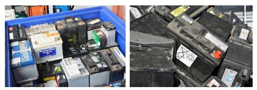
Figure 34: Appropriate and inappropriate storage of lead acid batteries
