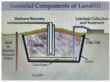
Figure 22: Schematic for landfill site
