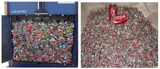
Figure 13: Compacted, baled, and shredded aluminium cans
